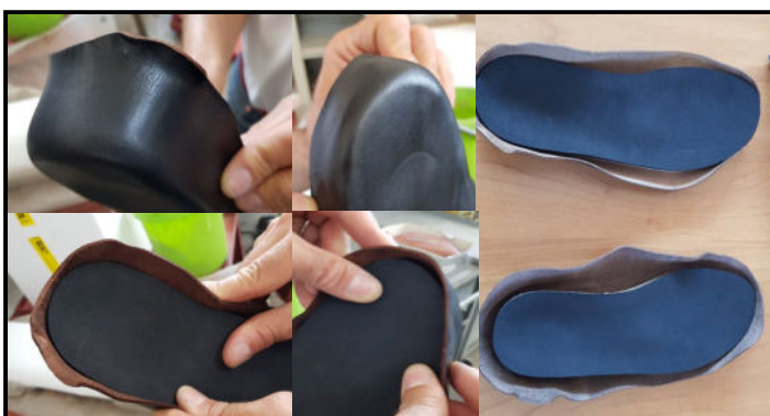
SAGOMATURA RICOPERTURA CEPPO SANDALO ARABO SHAPING OF THE COVER OF ARABIC SANDAL SOLE
